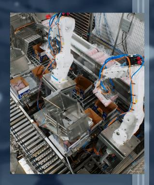
Deliver consistent results with precise case-packing robots. Save time during sanitation with washdown-ready designs. Avoid the headaches with turn-key automation tailored to your plant.
