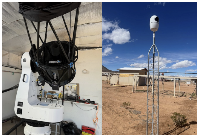
Figure 4: SW New Mexico Polaris Observatory- 0.5 meter Planewave telescope and L500 mount. To the right is the Beacon 8.0 PTZ for wide field acquisition
