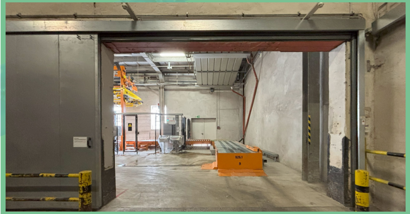
Figure: Fire door equipped with a protective barrier to prevent impact damage.
