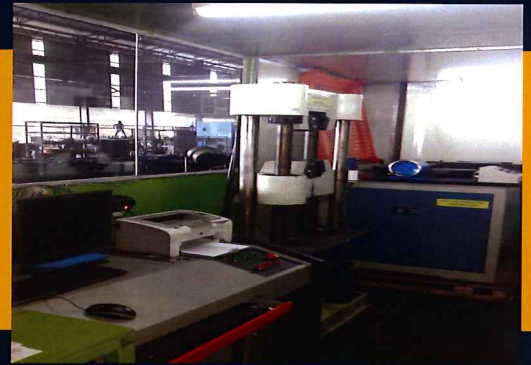
Tensile yield / strength / bending and rebending testing equipment
