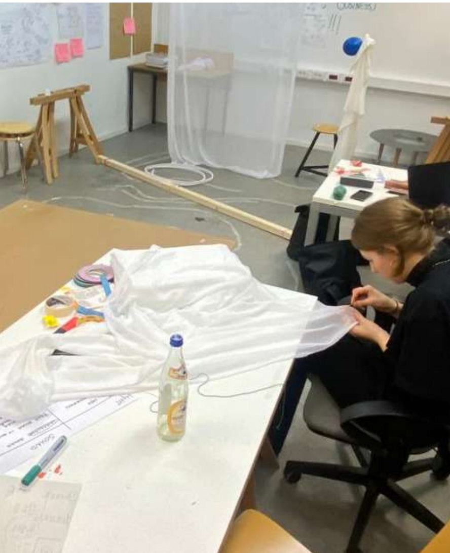
fig. 37 Placing the embroidery pattern, cotaining conductive thread, in the fabric.
