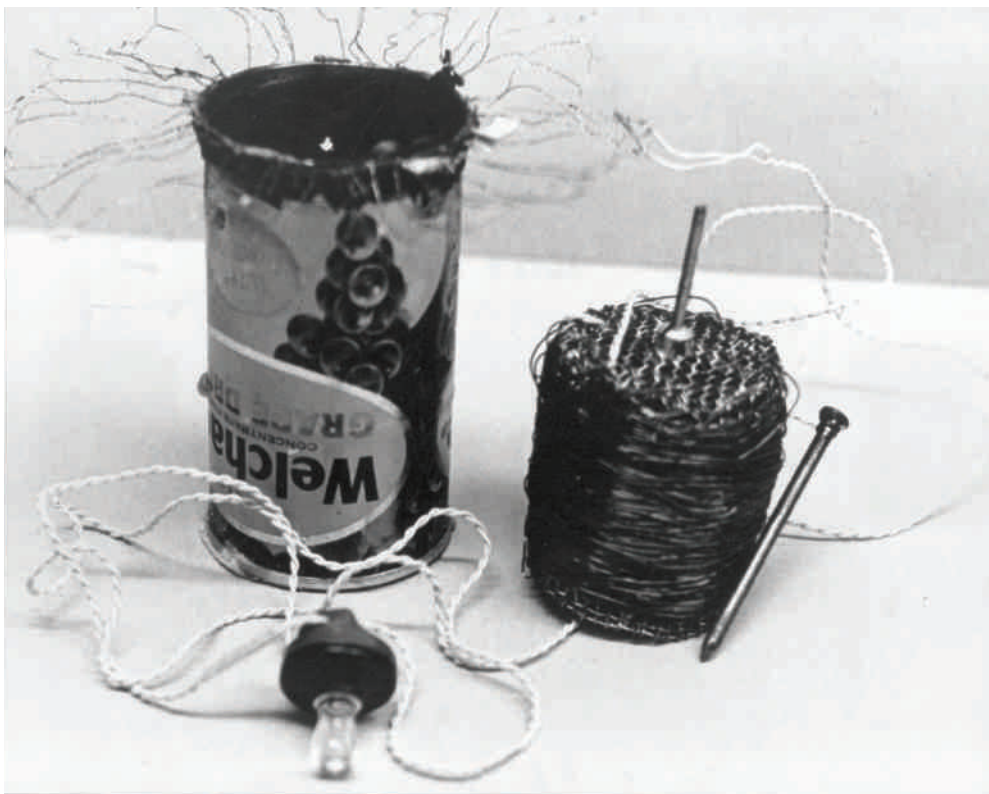
3.4 Tin Can Radio: radio receiver designed for use in the developing world at 9 cents a piece. By Victor Papanek and George Seeger at North Carolina State College. Originally published in Victor J. Papanek, Design for the Real World (New York: Pantheon Books, 1971), 163. Victor J. Papanek Foundation, University of Applied Arts Vienna
