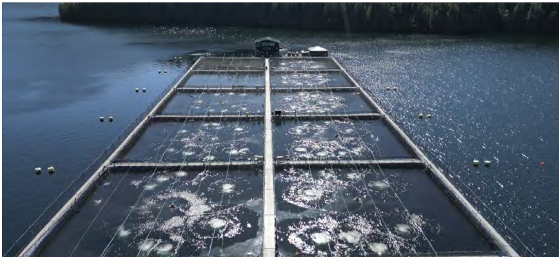
Figure 26. Innovation to reduce greenhouse gases: view of Poseidon's new Flowpressor™ aeration system, which slashes greenhouse gas emissions by 60% compared to conventional diesel compressors used to mitigate plankton blooms.
