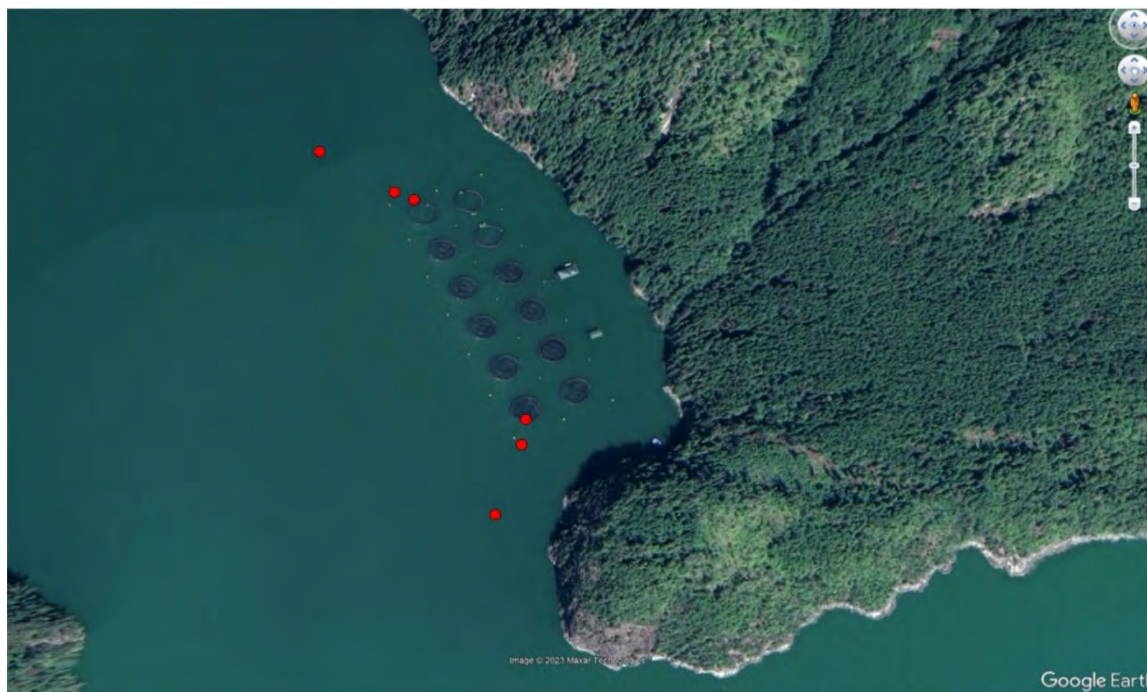
Figure 17. A typical two-transect monitoring survey design for a soft-bottomed site. Grab samples are collected at cage edge, 30 meters and 125 meters from the array along dominant and sub-dominant current directions. Note that cage arrays longer than 200 meters require more than two transects if perpendicular to the current flow.
