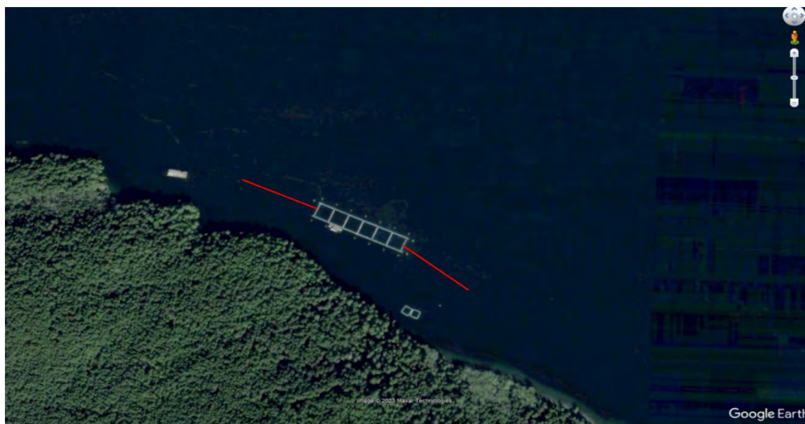
Figure 20. A typical two-transect underwater video survey design for monitoring a hard-bottomed site.
