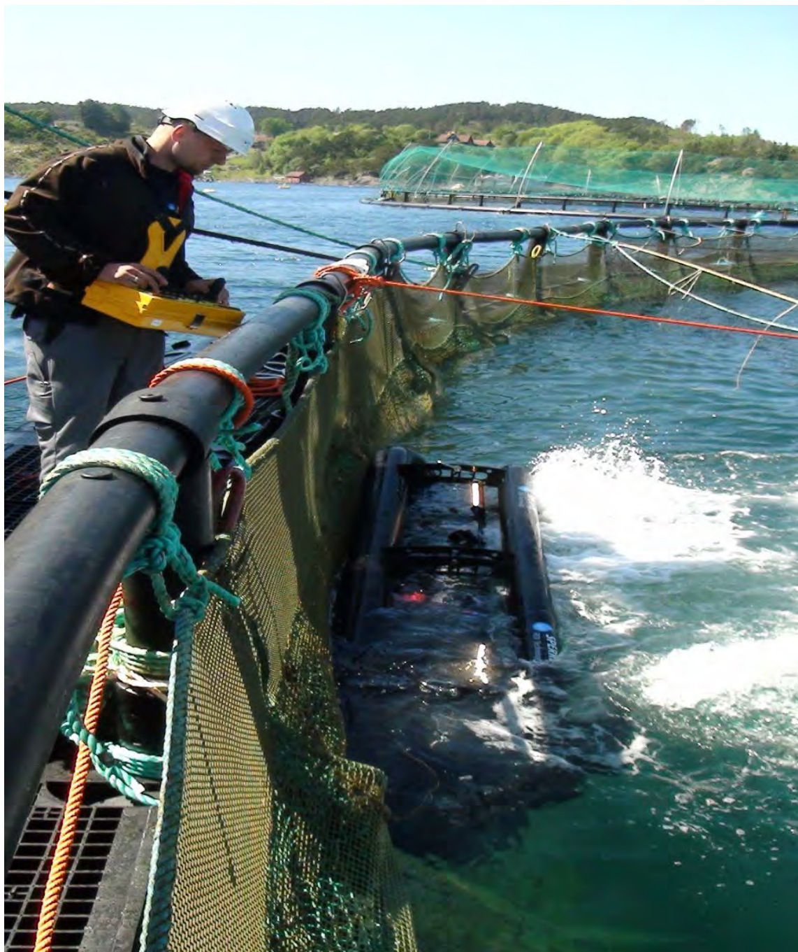
Figure 8. View of net scrubber in pen. Routine net cleaning prevents biofilm build up on nets and maintains water flow for salmon.
