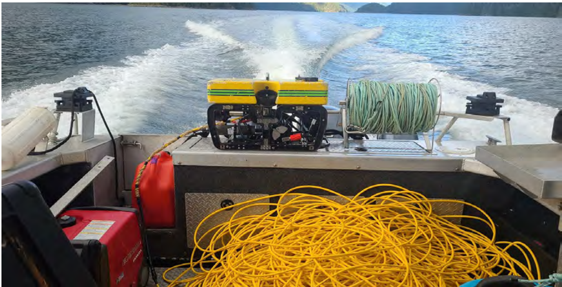
Figure 18. View of remotely operated underwater vehicle camera used to monitor “hard bottom” sites.
