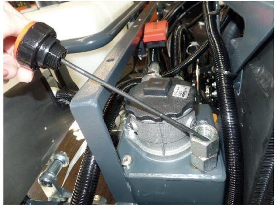
Always check the condition of all hydraulic lines and O-rings for leaks. For this purpose, a cardboard box can be placed underneath to detect any leaks. If leaks occur, replace the component to be replaced if it is defective or damaged.
