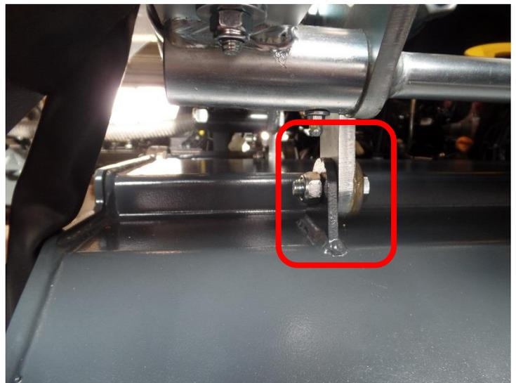
Mount the mounting tabs on the mulcher!!
