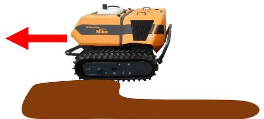
Do not move along the edge of a slope or uneven surface while one rubber track is in horizontal position and the other is tilted or partially raised.
