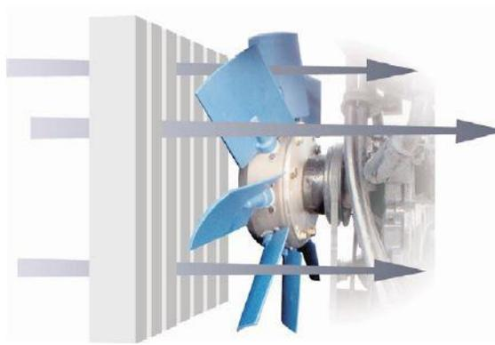
When the control switch is actuated, the blades change their angles as shown in Figure 2 so that the air is directed back through the cooler, which removes dirt and dust particles through the fan reversal. The operating unit allows the operator to carry out additional cleaning cycles in very dirty and dusty environments.
