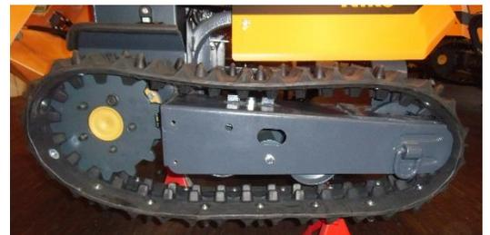
Pull the drive wheel teeth out of the track guide. The track is heavier than it appears. Do not try to carry their weight and it is better to let them fall to the ground.
