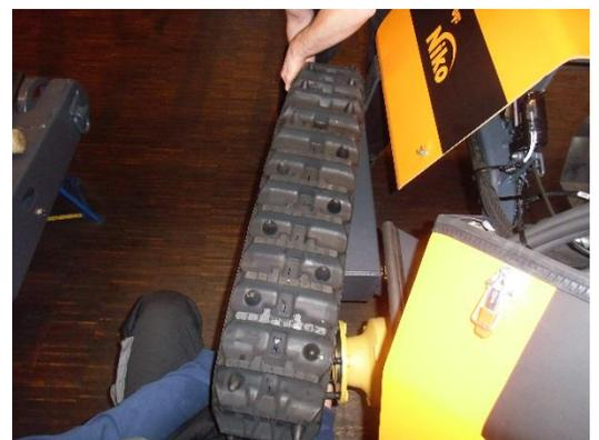
Re-tighten the 27 mm grease nipple, if necessary, replace the seal underneath and use the special grease gun supplied to pressurise the track tension cylinder. The pressure gauge on the grease gun must read 180 bar to ensure correct track tension.
