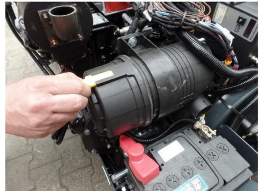
Pull the main cartridge out of the overall filter by turning it slightly.
