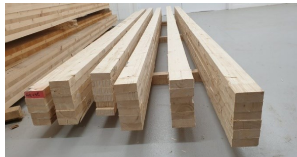
Completed GLT beams
