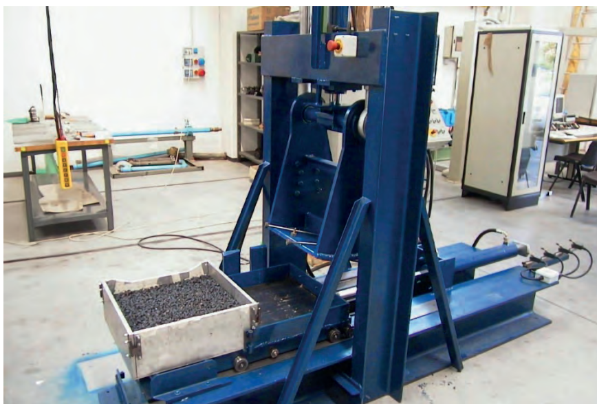
Figura 2 – Compattatore lastre in conglomerato bituminoso. Figure 2 – Asphalt mixtures slab compactor.
