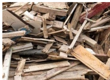
Figure 19. Treated and non-hazardous wood, mostly solid wood
