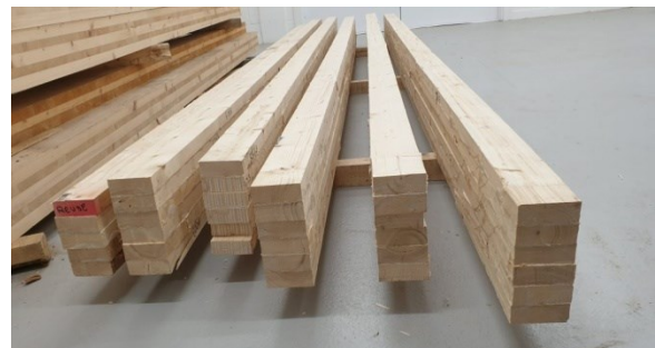
Completed GLT beams
