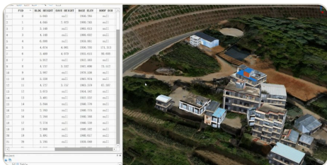
EVERY STRUCTURE WITH HEIGHT AND ELEVATION ATTRIBUTES
