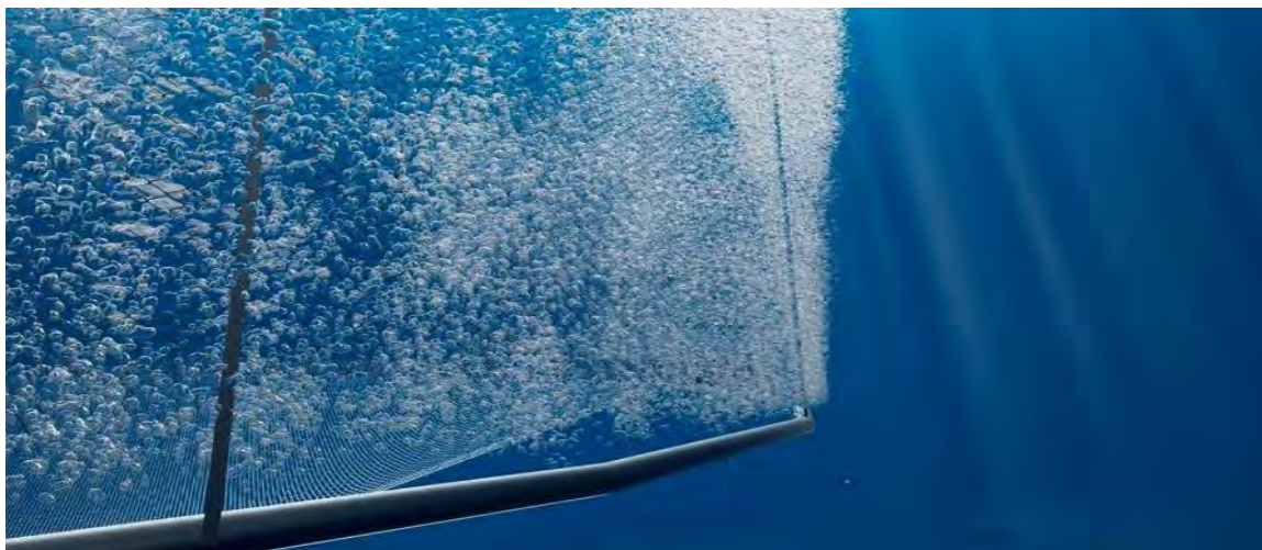
Figure 36. Aeration/bubble curtain deter sea lice from entering net pens.
