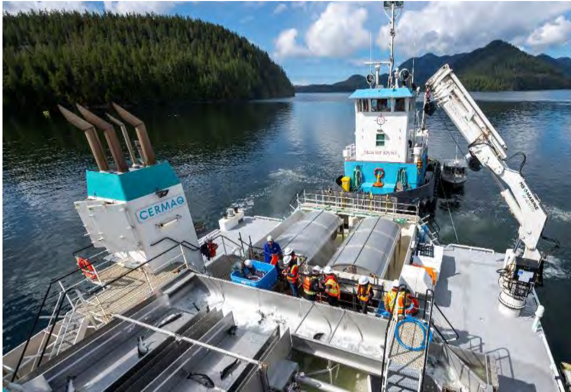
Figure 40. View of treatment vessel using low-pressure water to remove sea lice.
