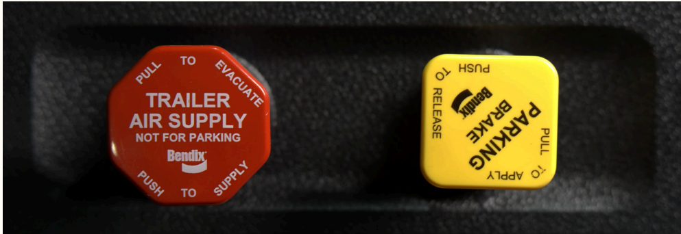
Figure 6: Air brake control panel
