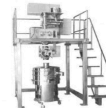
Processing Machine: Roll Compactor Control: PLC 21 CFR Origin: India
