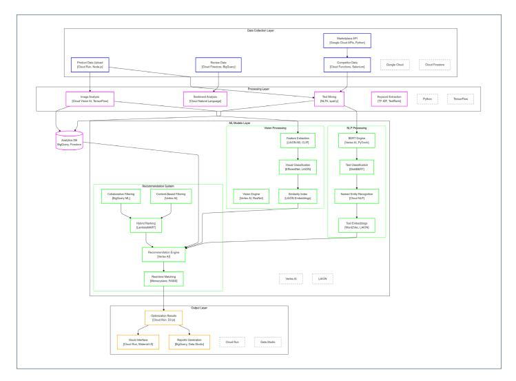
The PoC and further architecture patterns were architected as a modular microservices system deployed in Google Cloud Platform, utilizing containerized applications for maximum flexibility and scalability. The architecture consists of four distinct layers.
