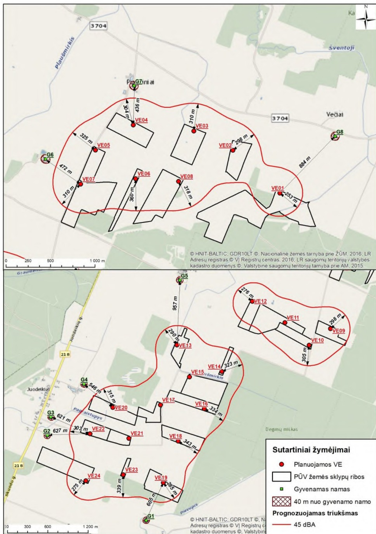
2.11.1 Fig. Isolines of the predicted noise level of the PŪV at a distance of 40 m from the nearest residential buildings.
