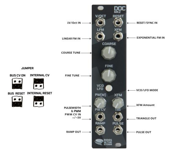
Discrete VCO with stabil tune and wide spectral range
