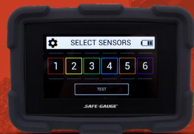
SafeGauge's hand-held MultiTool allows technicians to monitor and record multiple channels simultaneously - delivering significant productivity gains.
