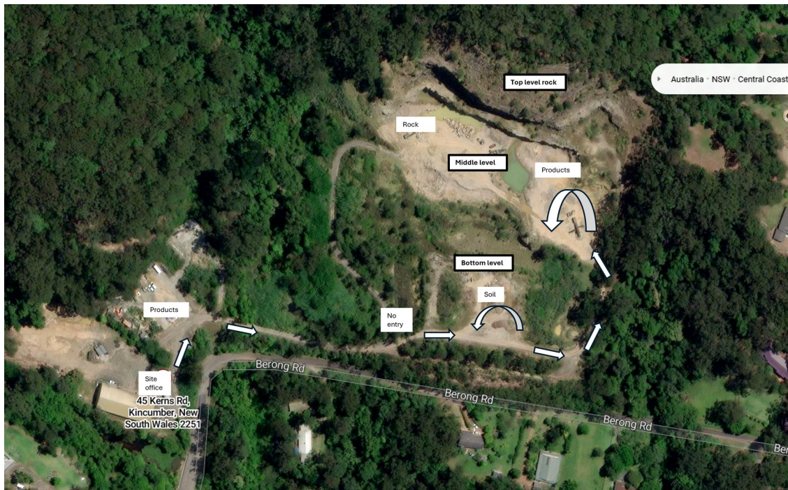
Kincumber Quarry — working areas, access and product storage.
