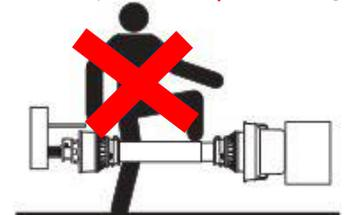
Friction clutches can reach very high temperatures during operation. Do not touch!
