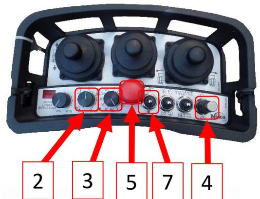
3.) Release the emergency stop button (5) on the transmitter (remote control) by turning the it clockwise
