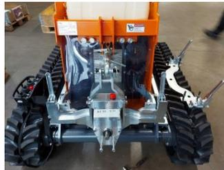
Hook in the Rapid holder & fold up the locking lever
