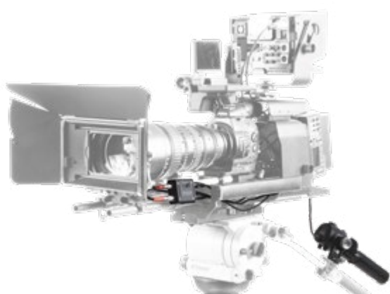
ENG SETUP WITH CANON BROADCAST CONTROLLERS AND NIPROS LS-750GT FOR IRIS CONTROL FROM THE OB-TRUCK
