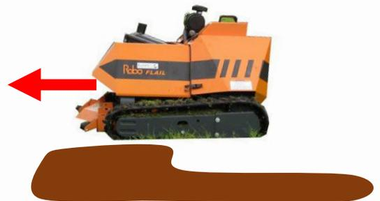
Do not move along the edge of a slope or uneven surface while one rubber track is in horizontal position and the other is tilted or partially raised.
