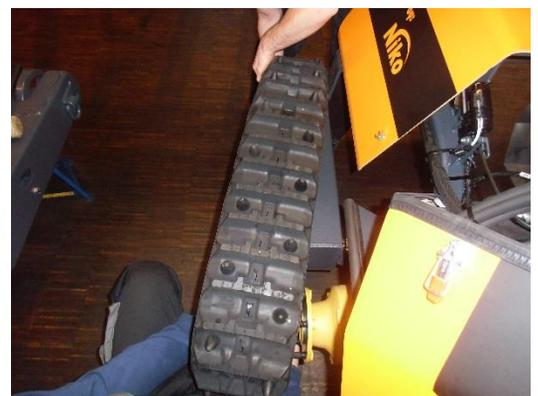
Re-tighten the 27 mm grease nipple, if necessary, replace the seal underneath and use the special grease gun supplied to pressurise the track tension cylinder.
