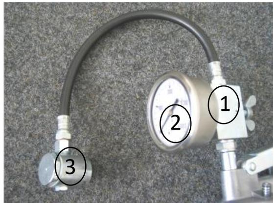
To relax, the grease nipple must be loosened until the necessary relaxation of the track becomes apparent.
