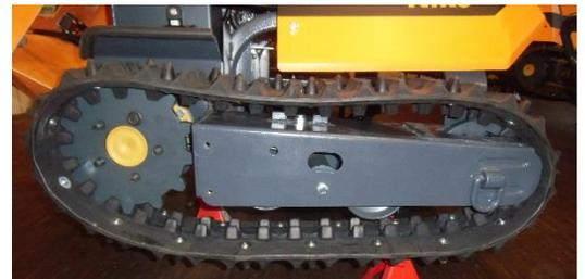
Place the new track to be installed on the guide rollers, then on the track wheel (pinion) while pushing in the top of the track.
