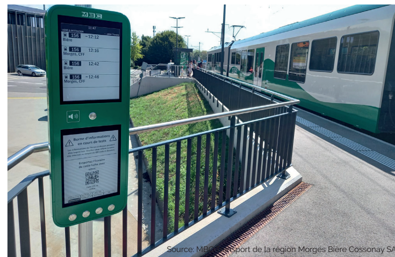
Source: MBO transport de la région Morges Bière Cossonay SA Double 13" iBus E-paper displays with 4 buttons and text-to-speech button, Morges, Switzerland
