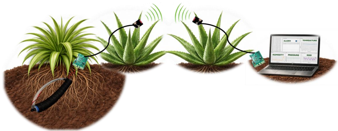
Figure 30. EcoSentinel PoC_v1 deployment diagram
