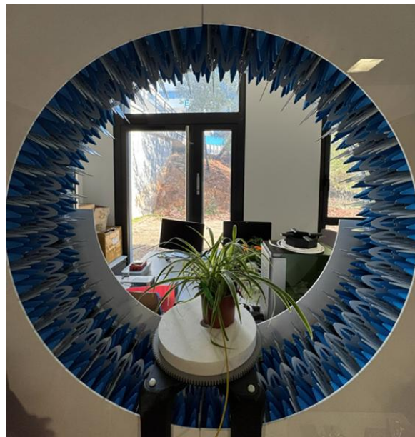
Figure 5. Measurement setup for measurement of radiation efficiency of plant-antenna booster on Chlorophytum comosum .
