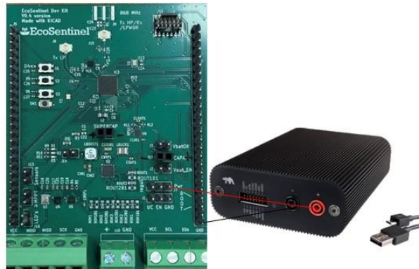
Figure 17. Setup Experiment 2 test 2 (power profiler and EcoSentinel Dev Kit).
