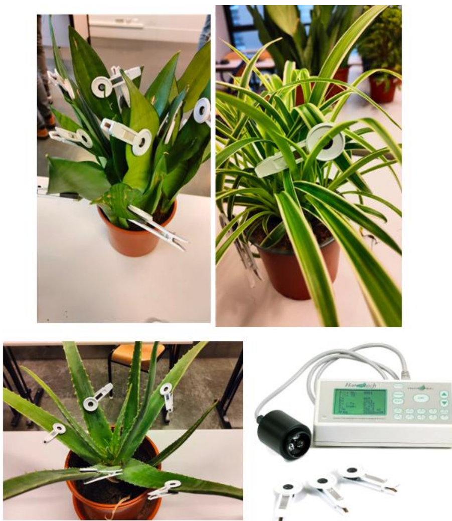
Figure 3. Experimental setup for measuring the fluorescence transient and photosynthetic efficiency. Leaves are dark-adapted using leaf clips (10 clips per leaf, in repeated measurements) for 30 minutes and then exposed to a 1-second pulse of photosynthetically active radiation. The signal is recorded by the Handy PEA and converted into a fluorescence induction curve, with simultaneous recording of photosynthetic efficiency parameters
