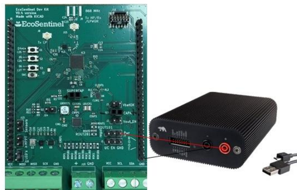
Figure 13. Setup Experiment 2, Test 1 (EcoSentinel Dev Kit and power profiler).
