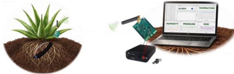
Figure 20. Setup Experiment 2, Test 3 (an EcoSentinel board sending sensor data to its gateway).
