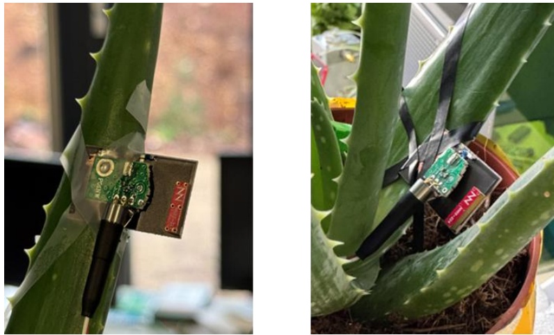
Figure 6. Antenna booster placement along the Aloe vera leaf: left, middle section of the leaf; right, lower section of the leaf.
