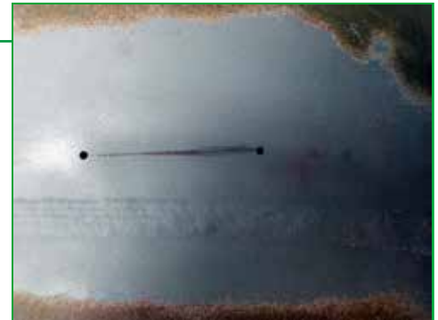
Abrasive blasting site showing leaks
