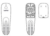
**Tips:** Use the tool to unscrew the four screws of the back cover.
