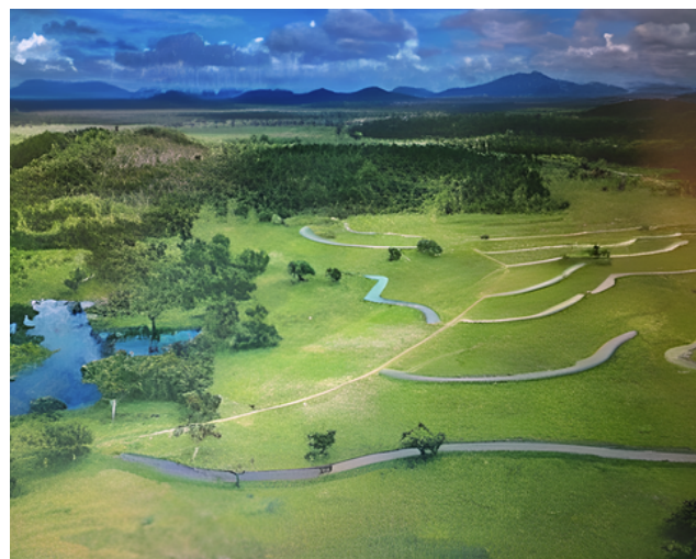
Figure 1. The rehydration swales collect water to rehydrate the soil.
