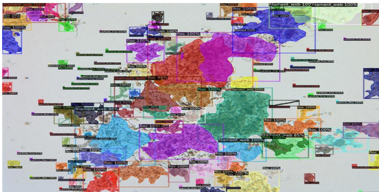
Flocmark® analysis result: flocs, filaments and fine particles are detected and measured in each image.
