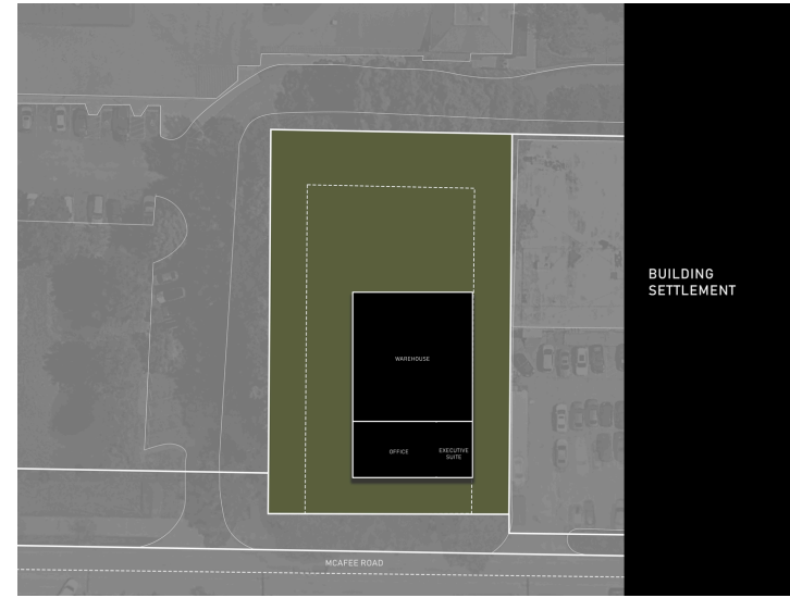
ZONING CONDITIONS ZONING DISTRICT C-1 FRONT SETBACK 0' SIDE SETBACK 20' REAR SETBACK 30' MAX LOT COVERAGE 80-90% OPEN SPACE 10% MAX BUILDING HEIGHT 35' TOTAL PARKING REQUIRED: 4 SPOTS / 1000 SQFT
