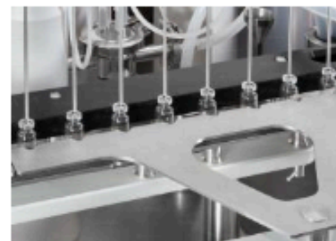
Processing Machine: Vial Filling Stopping & Capping Vaccines Control: PLC 21 CFR Origin: India
