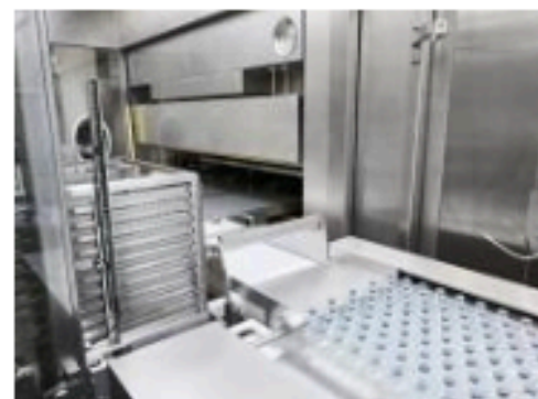
Processing Machine: Lyo with Auto Loading & Unloading System Control: PLC 21 CFR Origin: India
