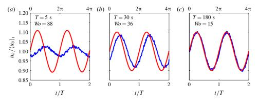
FIGURE 2. (Colour online) Normalized azimuthal velocity of the sinusoidally driven inner cylinder  $u_i/\langle u_i \rangle_t$  (solid red) and normalized azimuthal velocity  $u_\theta/\langle u_\theta \rangle_t$  at mid-gap (solid blue). Three Womersley numbers are shown, (a) Wo=88, (b) Wo=36 and (c) Wo=15. The velocity is radially averaged between  $0.3 \leqslant \tilde{r} \leqslant 0.7$ . On the top x-axis, we show the phase  $\Phi$  of the modulations in radians.
