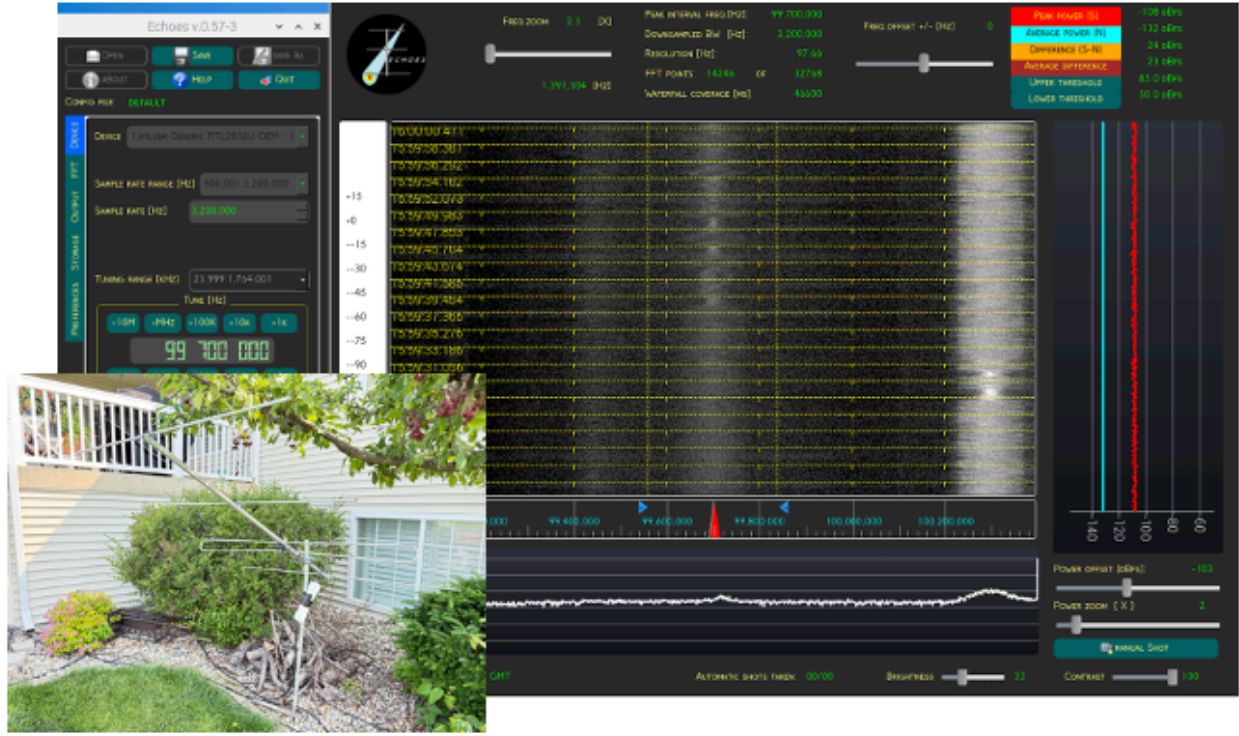
Figure 1. Echoes is experimental spectral analysis software, supported by an RTL-SDR and Yagi antenna, for the detection, counting and analysis of radio echoes produced by meteors entering the atmosphere. ( https://www.gabb.it/echoes/ )
