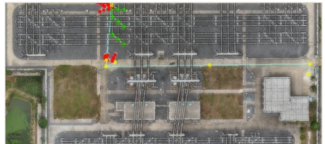
SUBSTATION ORTHOPHOTO WITH INSPECTION WAYPOINTS
