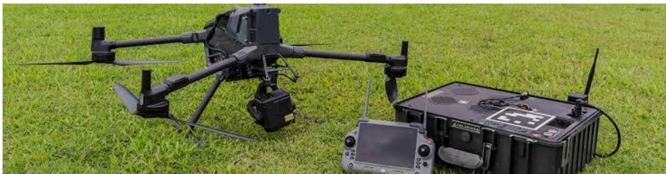
FIELD OPERATIONS. ENTERPRISE DRONE PLATFORM WITH RTK GROUND STATION, READY FOR A CAPTURE MISSION
