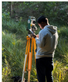
TOTAL STATION VERIFICATION IN THE FIELD
