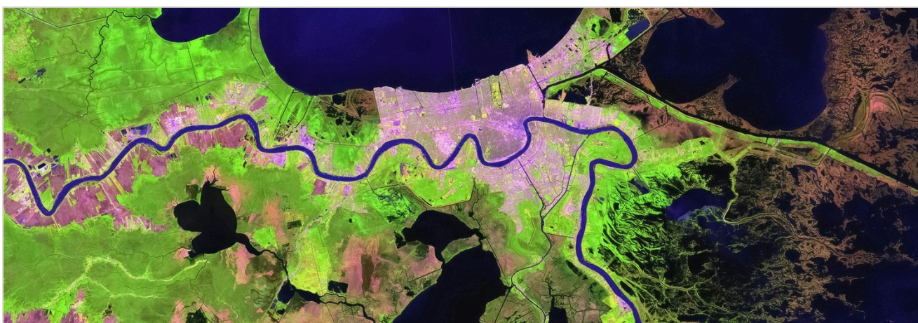
A RIVER DELTA IN FALSE COLOUR. VEGETATION, SEDIMENT AND OPEN WATER SEPARATED BY THEIR SPECTRAL SIGNATURES
