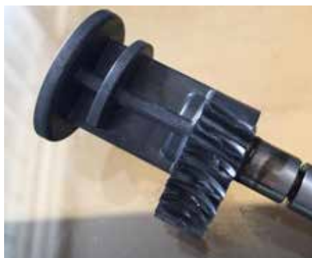
WORN ACTUATOR GEAR
