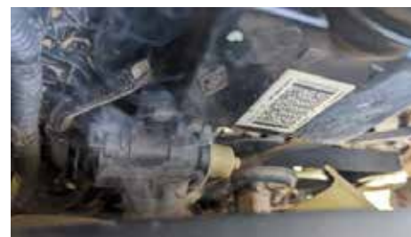
VSV SWITCH SMOKE TEST
