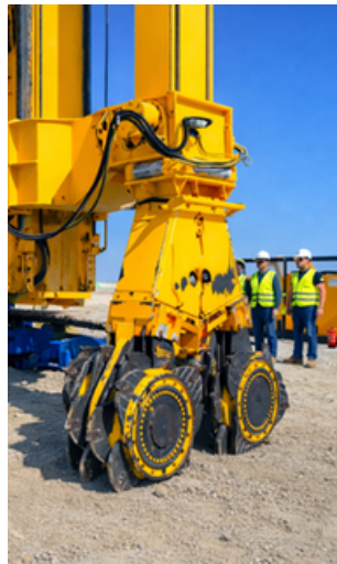
CSM Wall Installation Shafts for Storm Water Drainage Project – Qassim, KSA
