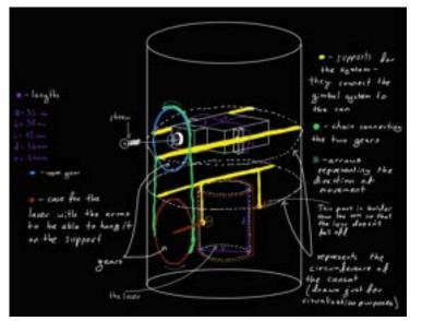
Fortunately, we have produced a way to simplify the gimbal in a way that it fitted into the Can. The idea involved only one 180-degrees-rotation servo motor which meant that the laser was going to be able to rotate only about the pitch axis. Here is a sketch of how our gimbal was going to look like:
