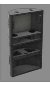
The Power side of our Can is much simpler. The semi-circular design will be outfitted with a flattenedout bottom, allowing for a multitude of mounting positions. Due to the gimbals design and dimensions, it will protrude out-side of the Payload side, therefore using the space leftover is a perfect location for the brains of our operation Raspberry pi Zero. This side will be outfitted with a shelf design where we will be able to stack components on top of one another by using "shelves".
