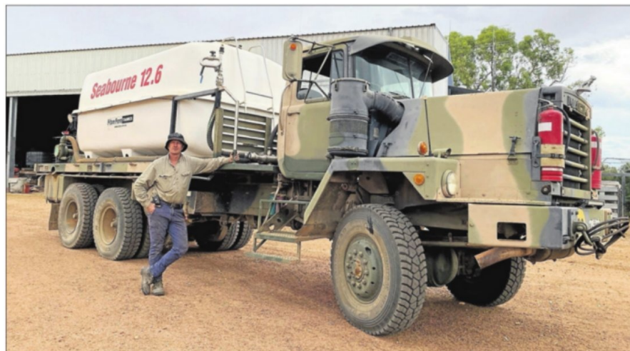
□ Tony Seabrook and his son John (pictured) designed and built a 12,000-litre, six-wheel-drive, heavy-duty firefighting unit from an old army truck. Photo by Tony Seabrook.
