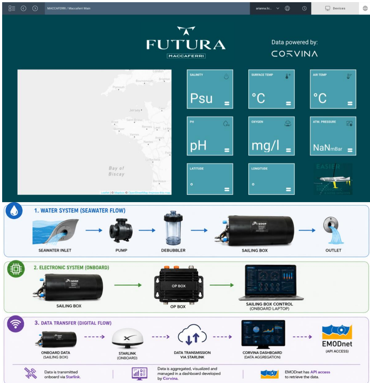
Figure 7. Maccaferri Futura onboard installation of the Sailing Box and data transfer via Navico OP Box to Corvina dashboard and EMODnet Physics.
