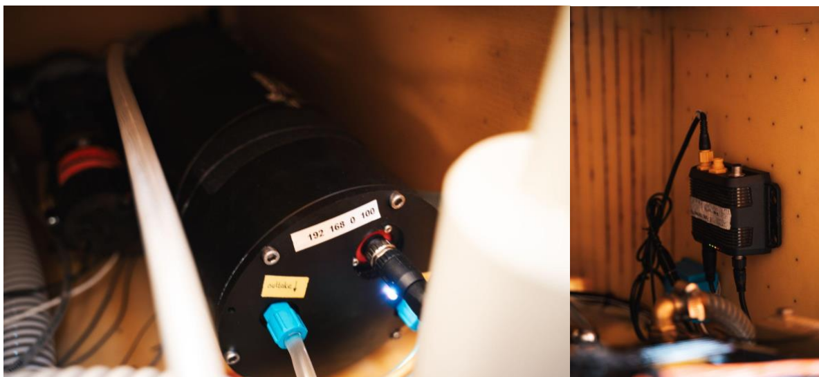
Figure 5. The Sailing Box low-cost device (left) installed onboard the Class40 Maccaferri Futura gathering seawater data, and the Navico OP Box (right) gathering navigational data and sharing all via Starlink connection
