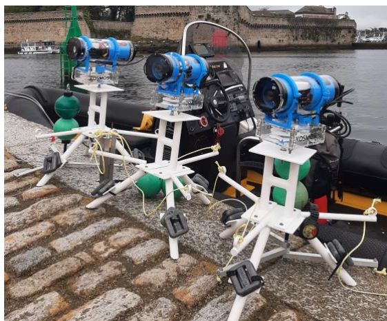
Figure 25. The KOSMOS lander (V4.0)(left) with example of image collected (right)
