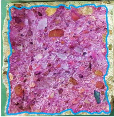
Figure 5. Appearance of a sample prepared for measuring carbonation depth after surface treatment with phenolphthalein solution
