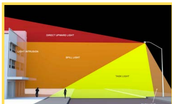
Figure 6 Light spill into nearby residences and upward into the sky produced by a street light (Source: Citelum, 2016)
