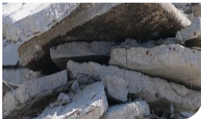
Oversized concrete pieces (OC)
