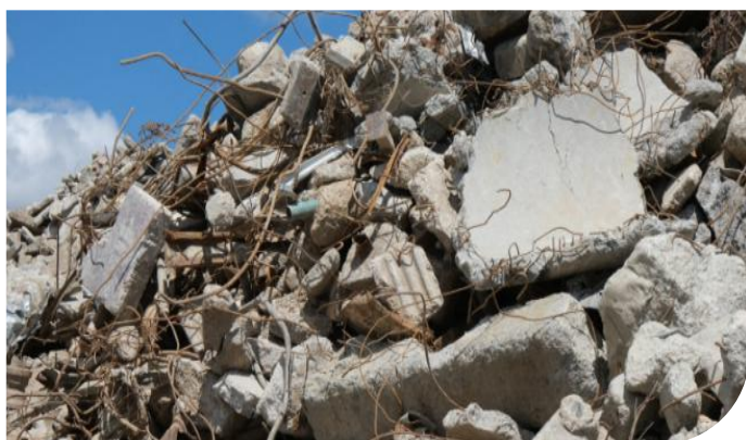
Clean and sorted concrete (CSC)
