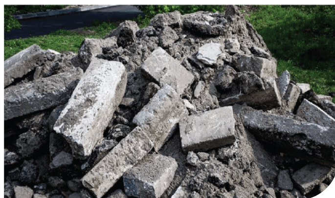
Concrete and dirt (CD) without plastic or timber
