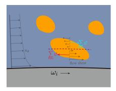
FIGURE 6. A sketch of how the interfacial tension works in a TC system.
