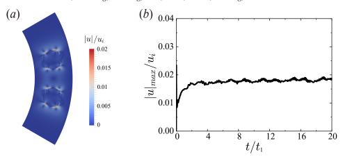
FIGURE 12. Spurious currents for two static drops in a TC system with the two cylinders fixed. (a) Contour of the velocity magnitude. (b) The maximum velocity magnitude,  $|u|_{max}$ , as a function of time.  $|u|_{max}$  is normalized by the velocity of the inner cylinder  $u_i$  considered in our work and the time t is normalized by the time required for one full rotation of the inner cylinder  $t_1 = 2\pi r_i/u_i$ .
