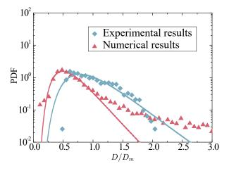
FIGURE 10. The PDF of the droplet diameter D with respect to the average diameter  $D_m$  for two-phase turbulence with  $\phi = 40\%$ . The solid lines denote the fitting results with a log-normal distribution function. The simulated results are compared with experimental results from our previous work (Yi et al. 2021).
