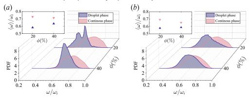
FIGURE 11. Angular velocity probability density functions for the droplet and continuous phases at the radius cut  $(r_{cut} - r_i)/d = 0.02$  obtained using (a) the standard VOF method and (b) the modified multi-marker VOF method. The inset shows the average angular velocity of the droplet and continuous phases.
