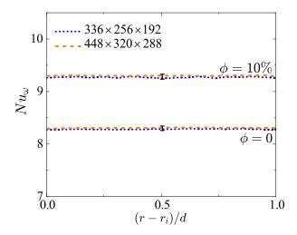
FIGURE 9. Radial dependence of  $Nu_{\omega}$  for two different grid resolutions. An error bar indicating a 1% error is provided for reference and both the cases for  $\phi = 0$  and  $\phi = 10\%$  lie within the error bar.
