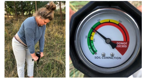
Above: Assessing soil compaction with a penetrometer.
