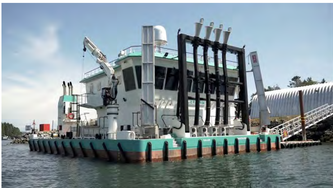
Figure 31. Veterinary practices are supported by specialized equipment, such as the hydrolicer barge shown above that removes sea lice with water jets.
