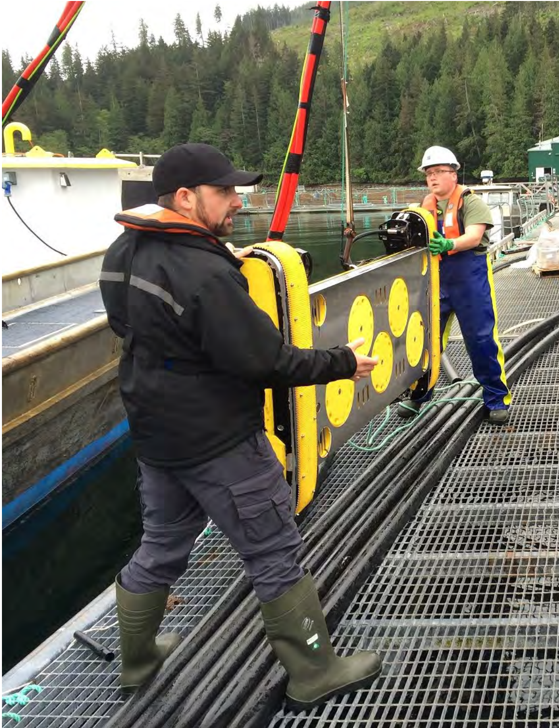
Figure 27. Net cleaning devices are used to keep containment nets clean to maximize water flow for fish health.
