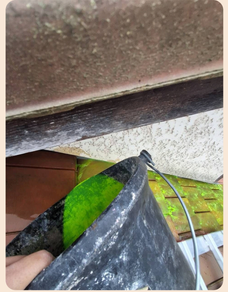
Test traceur UV fluorescent
