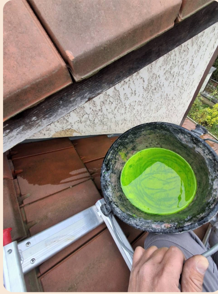
Test traceur UV fluorescent
