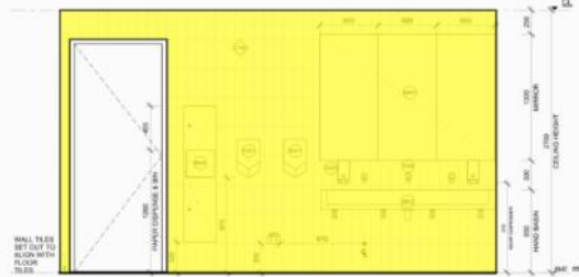
2 FEMALE TOILET - ELEVATION A 1:20
